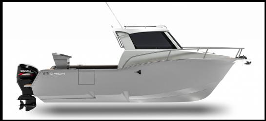
L.O.A 8.10m / Beam 2.50m / Fuel 450L/ Ballast tank 450L / 6mm Hull / 5mm Sides
