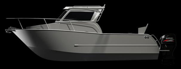
L.O.A 8.10m / Beam 2.50m / Fuel 550L / 6mm Hull / 5mm Sides
