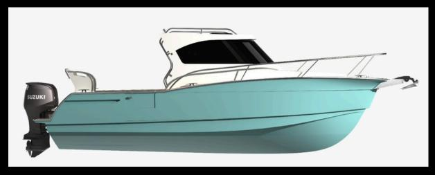
L.O.A 8.60m / Beam 2.89m / Fuel 850L/ Ballast Tank 800L / 6mm Hull / 5mm Sides
